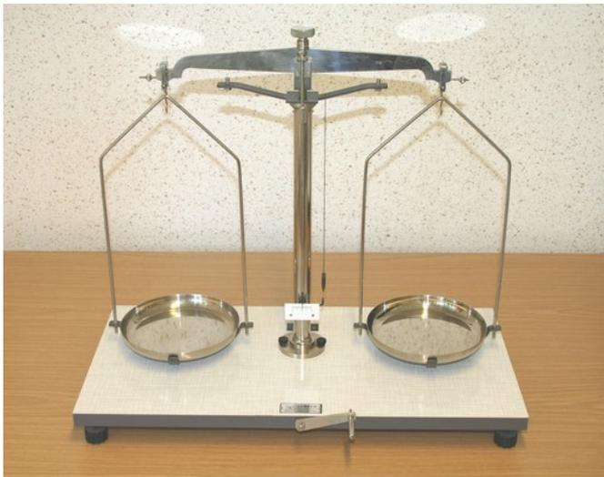
Fig. 2.11: Balkenwaage
