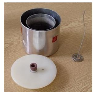
Fig. 7.21: Kalorimeter
